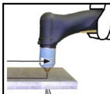
8. When ending a cut, the torch switch should be released and the torch lifted off the workpiece immediately upon completion of the cut. This is to prevent the pilot arc from re-igniting after the cutting arc has extinguished and causing damage to the nozzle (double arcing).
