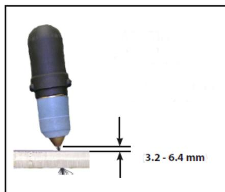
5. Depress the torch switch. Air should flow from the torch nozzle.
